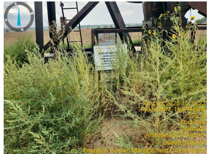
Photo 2 Wellhead sign partially covered with vegetation.
