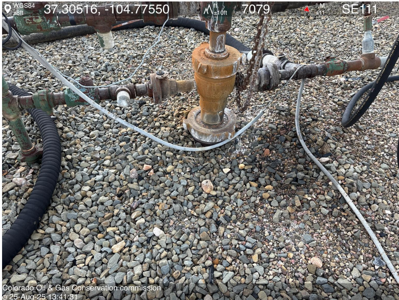
PHOTO 8: Bradenhead inaccessible. Install appropriate fittings to allow bradenhead visual inspection as per Rule 419.a.(1), (2) THIS IS THE SECOND NOTICE FOR THIS CORRECTIVE ACTION, IMMEDIATE ACTION IS REQUIRED.
