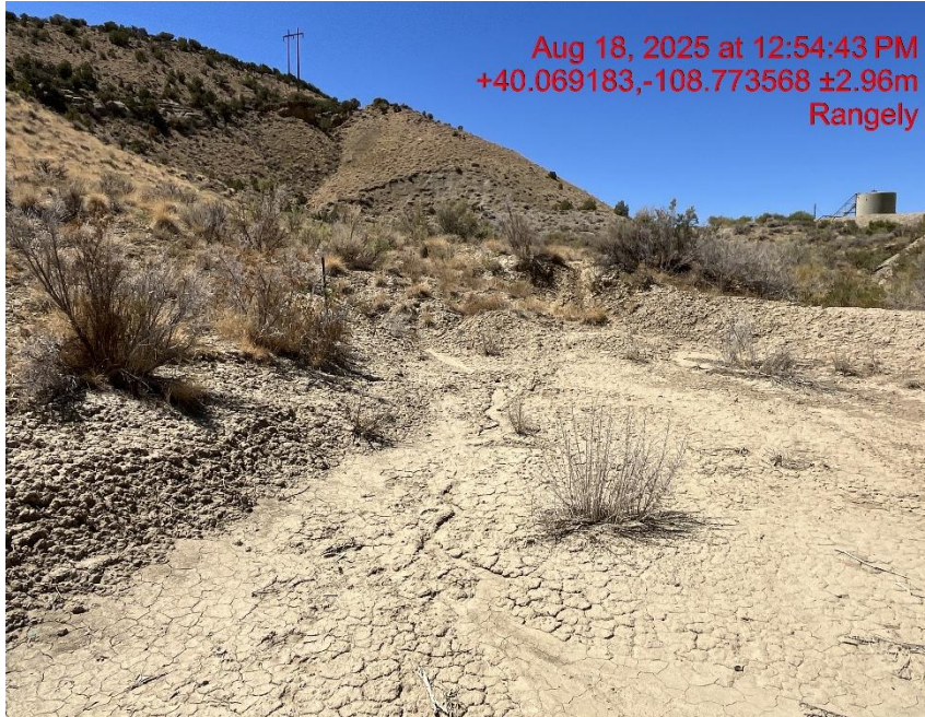
Photo # 2121 Failure to minimize erosion & transport of sediment onto location/insufficient BMP's
