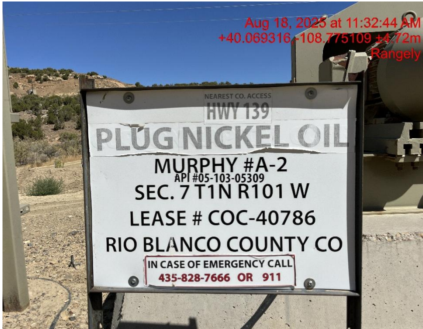
Photo # 2051 Wellhead sign lacks quarter/quarter section information. Additionally operator label is peeling but still legible.
