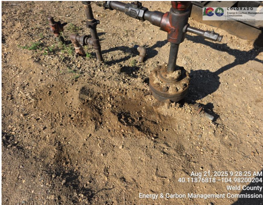
Stained Soil. Appears operator only placed clean dirt over the top of the stained soil.
