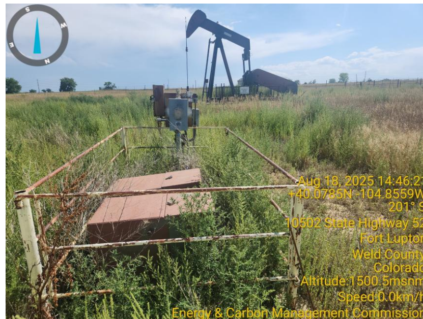
Photo 2 Well site, ancillary equipment overrun with tall vegetation.
