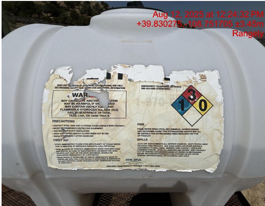
Photo # 1794 Chemical tank lacks required labeling & contains inaccurate operator information
