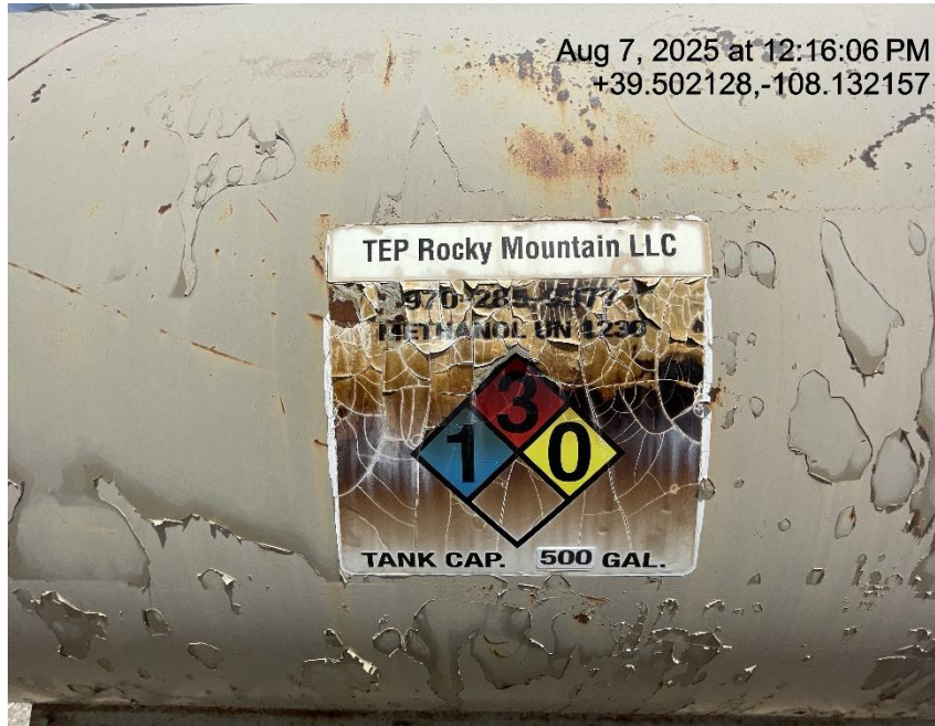
Photo # 9193 Tank label on methanol tank weathered, cracking & starting to become illegible
