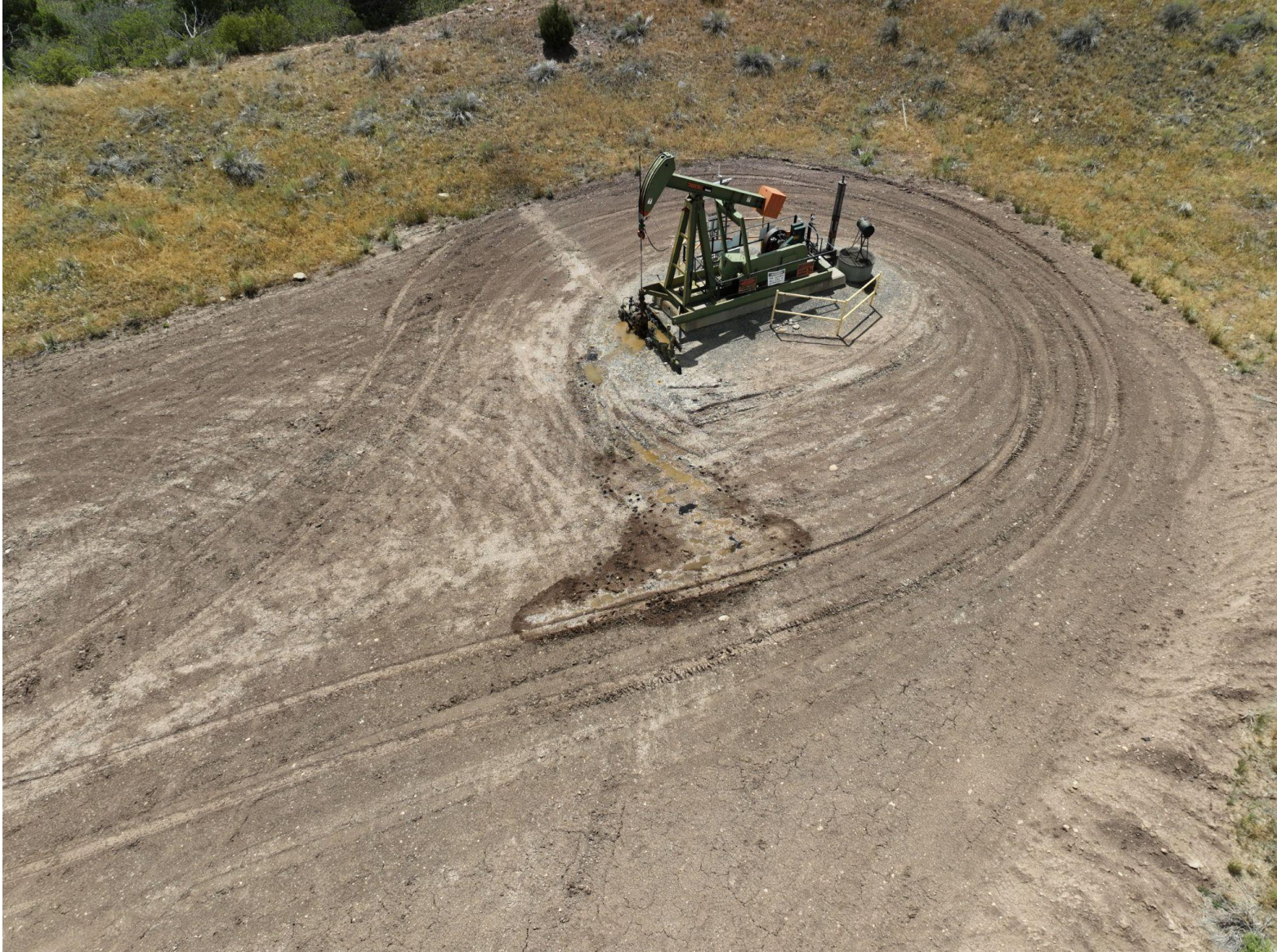
Photo 5. Drone photo showing extent of active spill.
