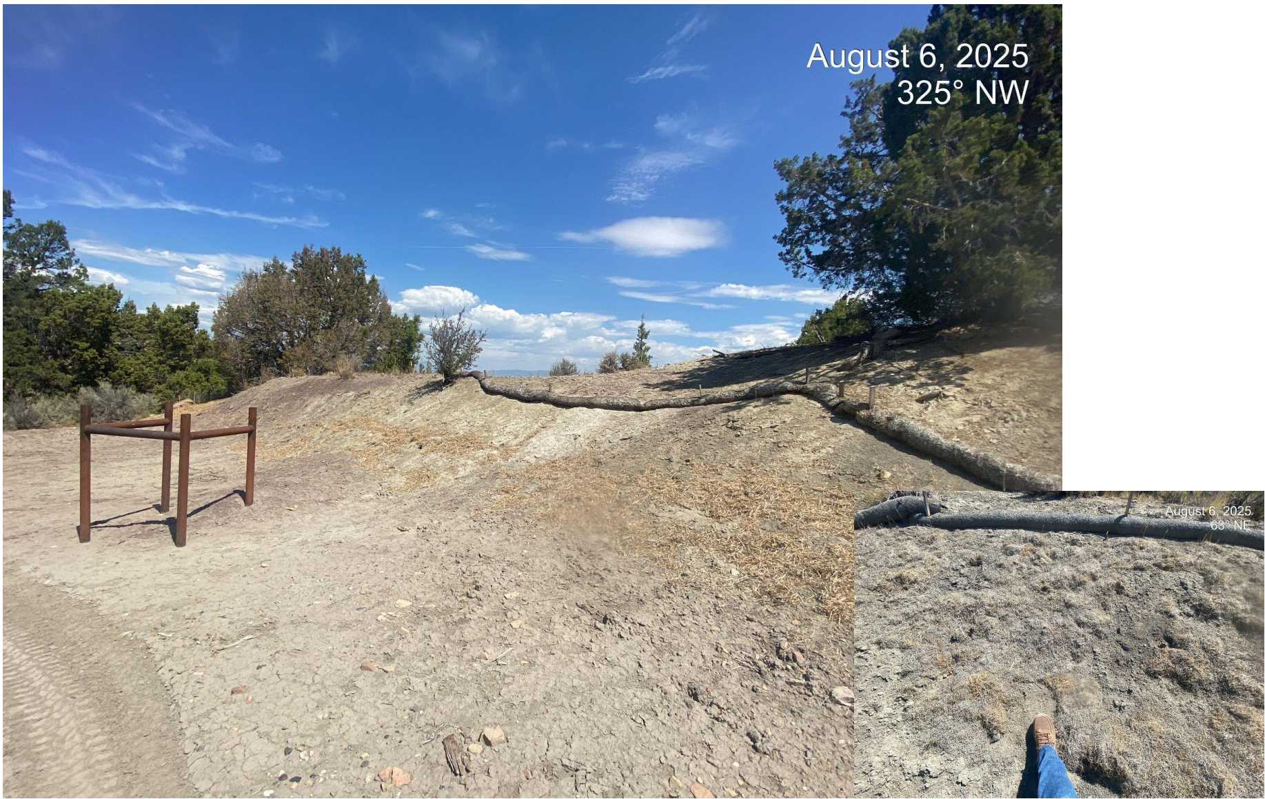
Photo 4. View of northern cut slope with perimeter stormwater BMPs. Operator appears to have seeded recently, no germination of vegetation was observed. Area remains with loose, bare soils.
