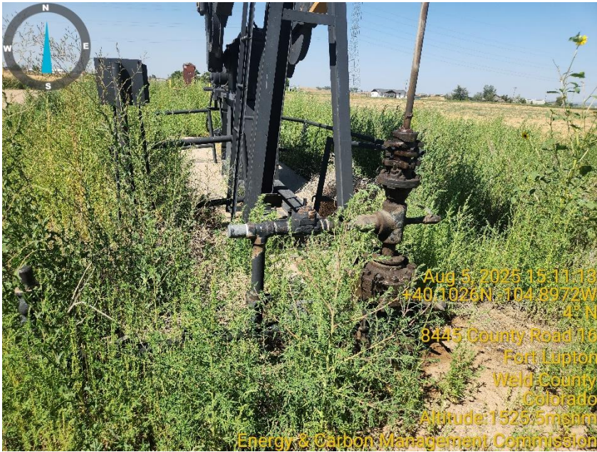
Photo 3 Wellhead in tall vegetation.
