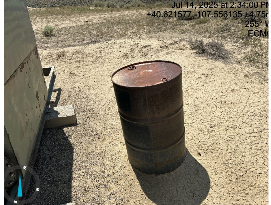
Unmarked drum not contained
