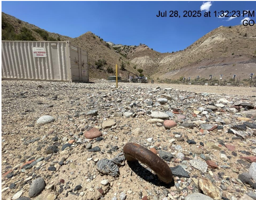
Photo # 5243 Unmarked deadman
