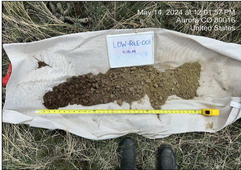
1. LOW-RtE-001 Soil Test Pit.
