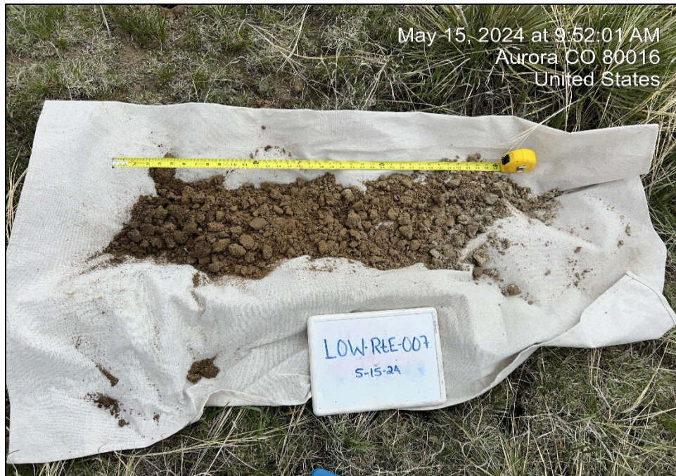
7. LOW-RtE-007 Soil Test Pit.
