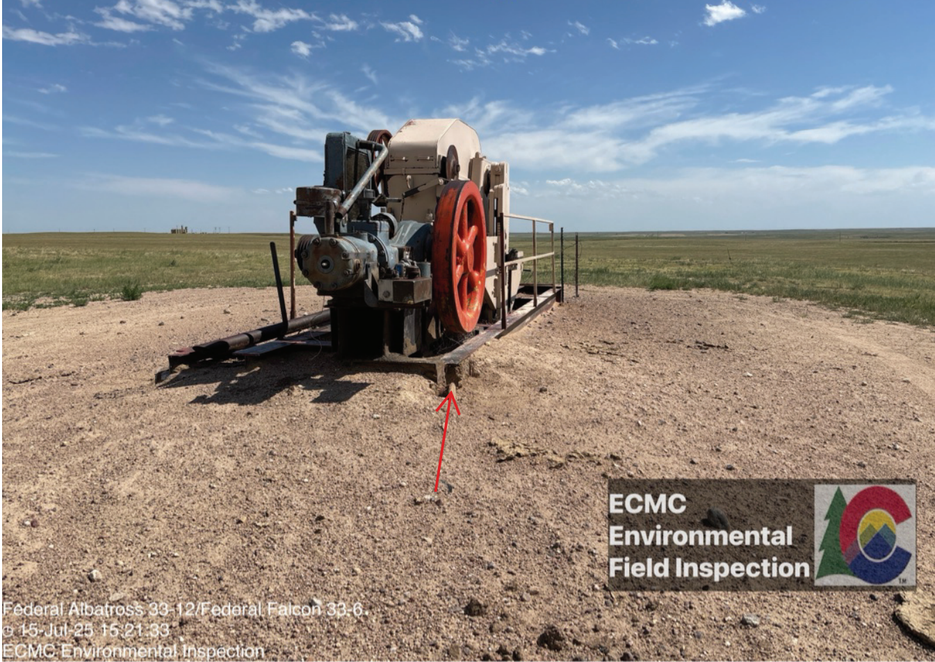
Stained soil adjacent to pumping unit at Federal Albatross #33-12 Well (API 123-20232)
