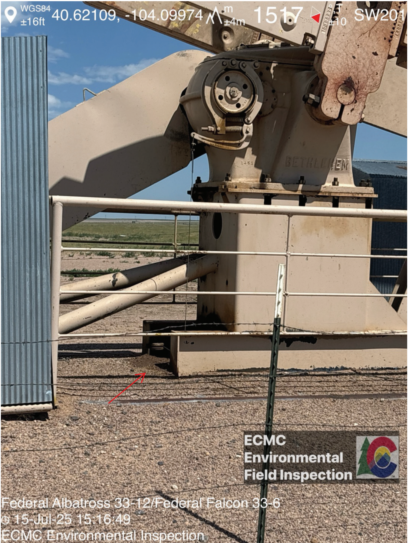
Stained soil beneath pumping unit at Federal Falcon #33-06 Well (API 123-20233)
