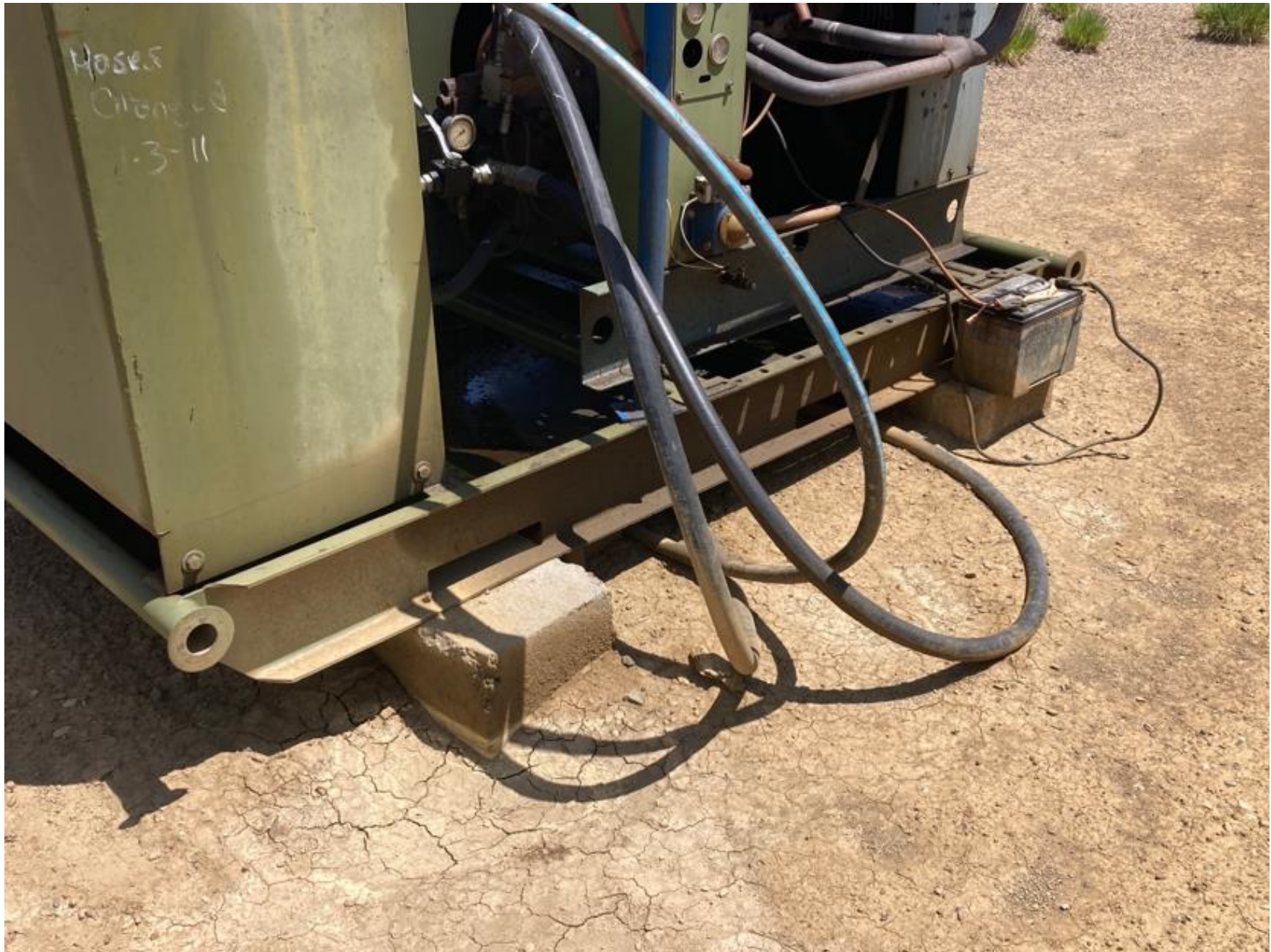
PHOTO 2: THE OILY FLUIDS HAVE BEEN REMOVED FROM THE ENGINE SKID AND MECHANICAL MAINTENANCE HAS BEEN PERFORMED. THE SELF INSPECTION PROCESS HAS BEEN REVIEWED.
