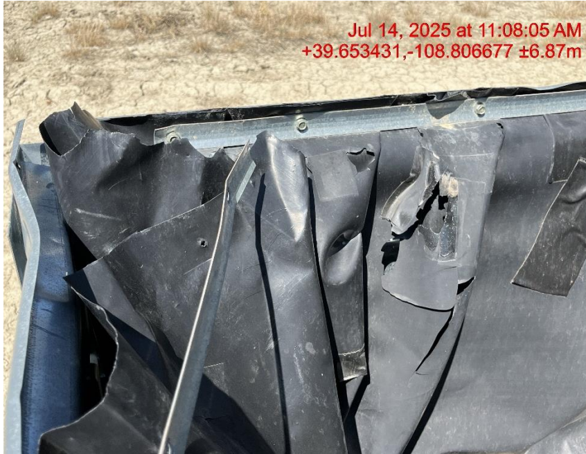
Photo # 9779 Multiple holes/tears in secondary containment liner/liner needs maintenance/liner lacks integrity
