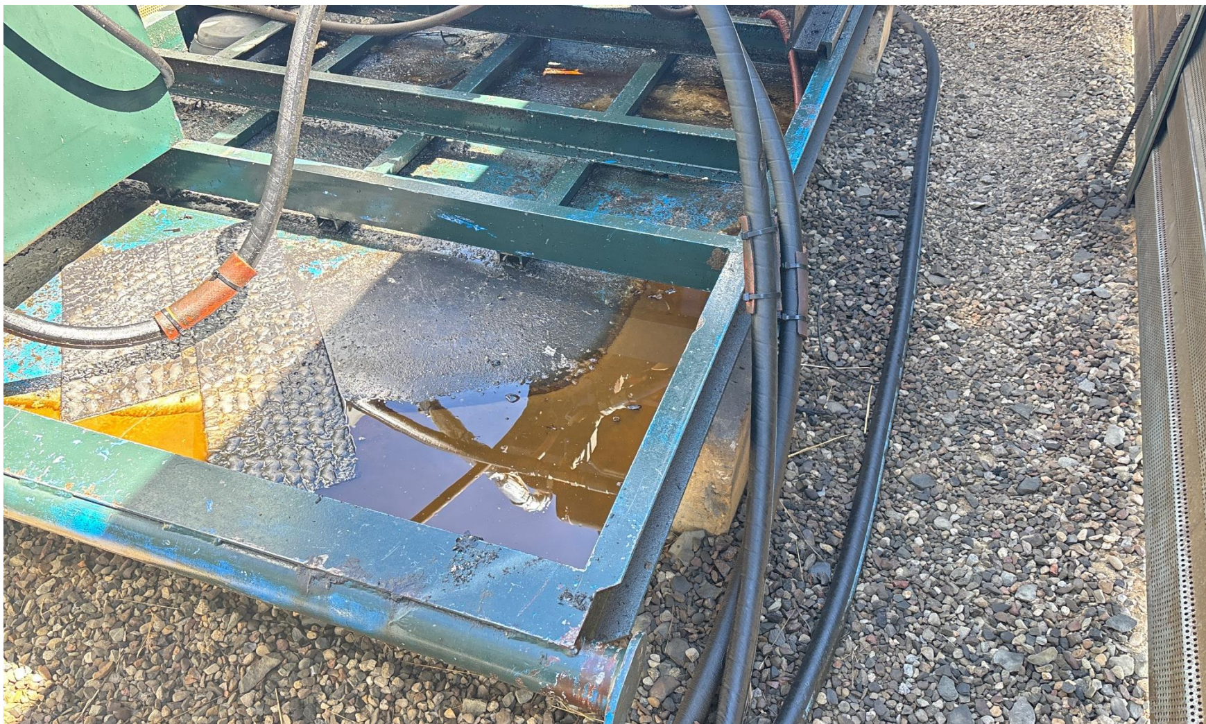
PHOTO 7: OILY WASTE IN PRIME MOVER ENGINE SKID. DRAIN OILY WASTE REPAIR ALL LEAKS AND REMOVE IMPACTED SOIL PER RULE 1002..(2).D & 1002.f.(2)B, Comply with general provisions of the oil and gas act for wildlife protection AND SB-181. 24 OURS TO DRAIL OILY WASTE. CA DATE 7-14-2025.
