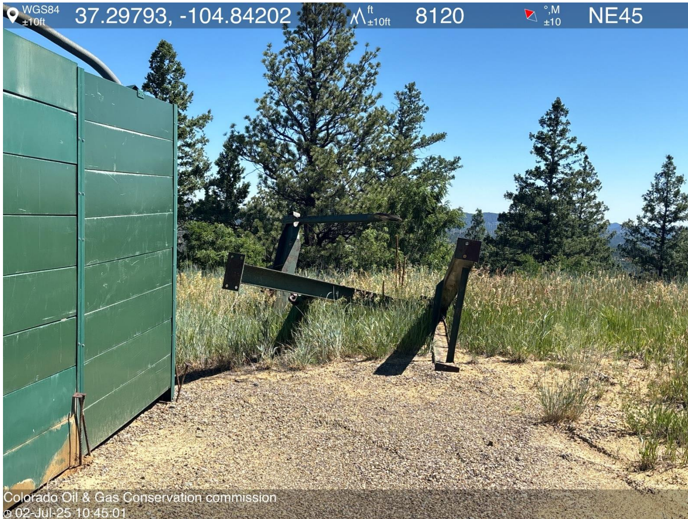
PHOTO 5: UNUSED EQUIPMENT (PUMPJACK AND ALL ITS COMPONENTS INCLUDING CEMENT PAD). REMOVE UNUSED EQUIPMENT PER RULE 606. CA DATE 7-14-2025.
