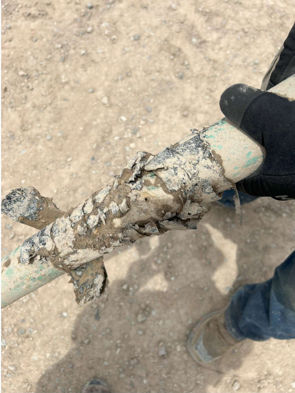
H17 (4A-16) flowline release point
