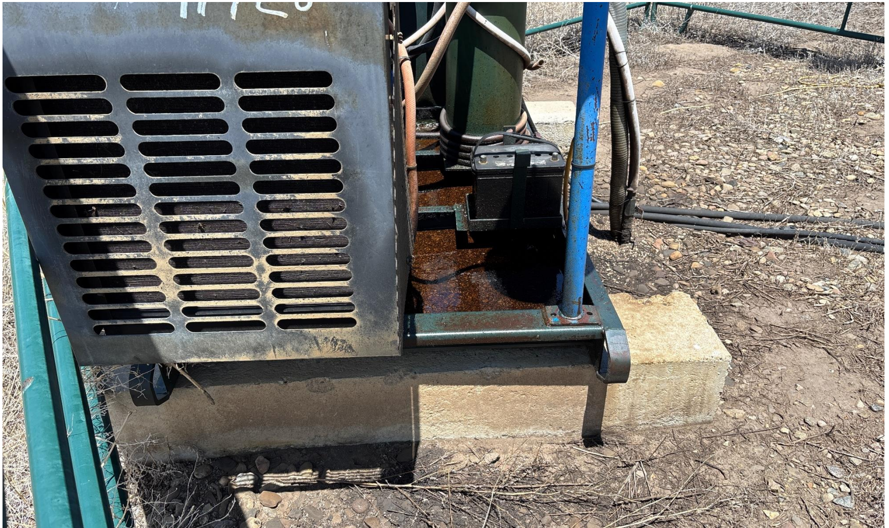
PHOTO 7: OILY WASTE IN PRIME MOVER ENGINE SKID. DRAIN OILY WASTE REPAIR ALL LEAKS AND REMOVE IMPACTED SOIL PER RULE 1002..(2).D & 1002.f.(2)B, Comply with general provisions of the oil and gas act for wildlife protection AND SB-181. 24 HOURS TO REMOVE OILY WASTE CA DATE 7-12-2025.
