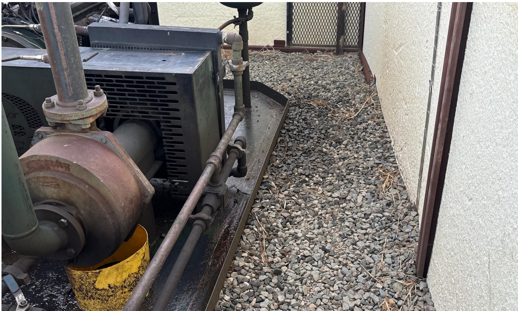
PHOTO 4: There is oil stained soil at the engine compressors and in the skids. Conduct maintenance on equipment, cleanup stained material and review self inspection processes. Conduct maintenance on equipment, FIX OR REPLACE LEAKING EQUIPMENT cleanup stained material and review self inspection processes. CA DATE 7-27-2025.
