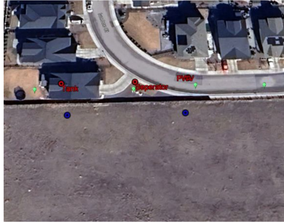
Photo 11. Google earth aerial imagery with the same markers as photo 10. It does not appear that the existing monitoring wells are associated with the remediation project.
