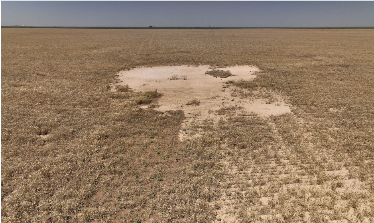
Photo 1. Drone aerial photo facing west toward the former wellsite. There is no crop growth at the ~100'x70' bare area.
