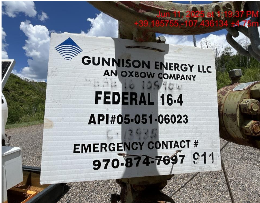
Photo # 8325 Emergency Contact Number is not in service, additionally quarter/quarter section is becoming illegible
