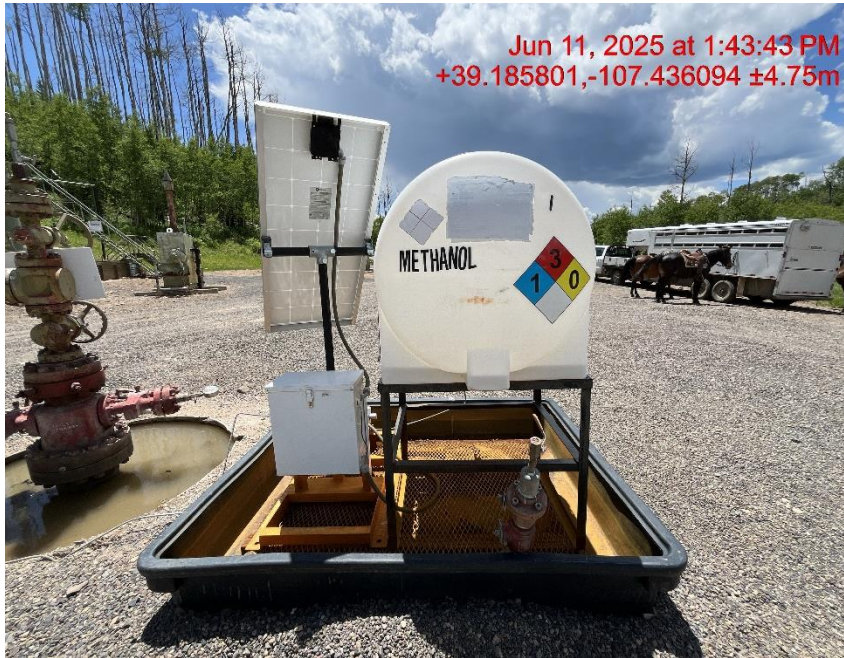
Photo # 8354 Chemical tank lacks required labeling/not in compliance with CECMC rules
