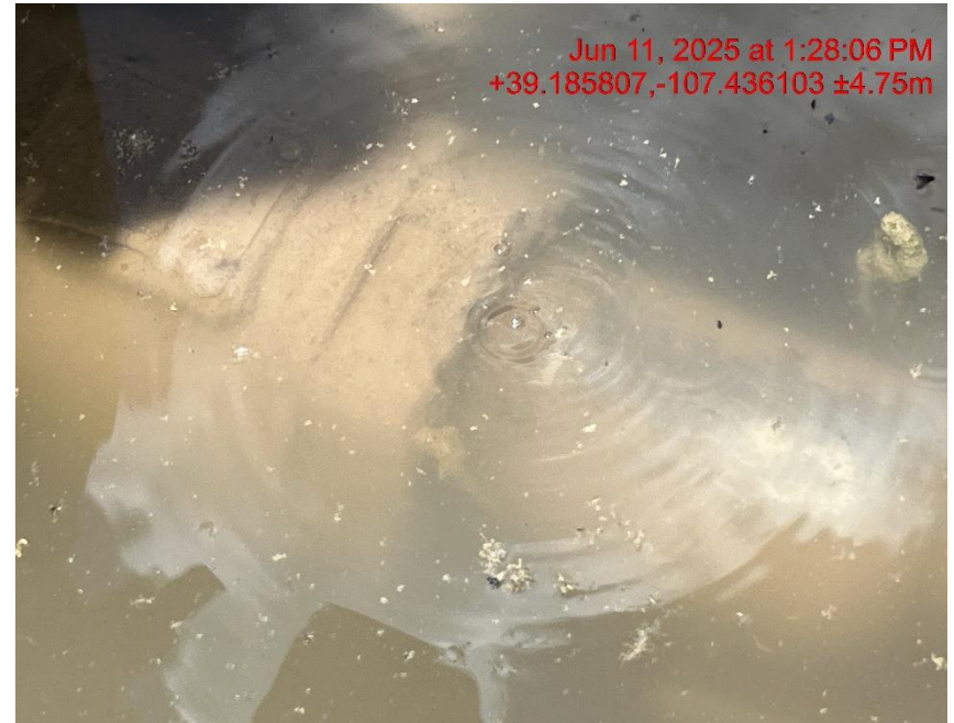
Photo # 8330 Bradenhead leak
