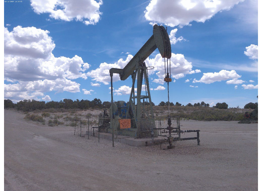
Pump Jack on producing well
