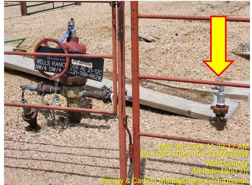
Photo 4 – Wellhead – Unmarked Riser
