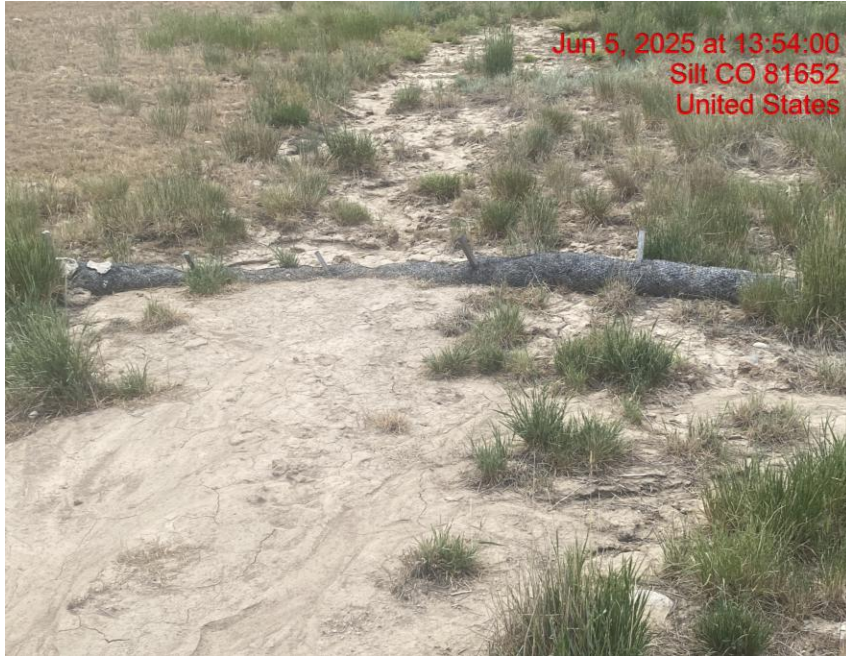
BMP Failure/Transport of Sediment Offsite – Photo #09169
