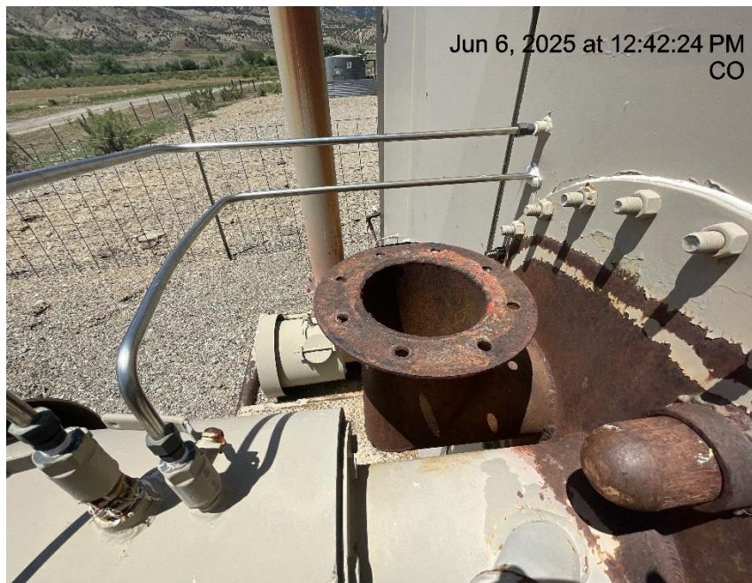
Photo # 7708 Burner exhaust open ended/wildlife hazard/available for entry by wildlife
