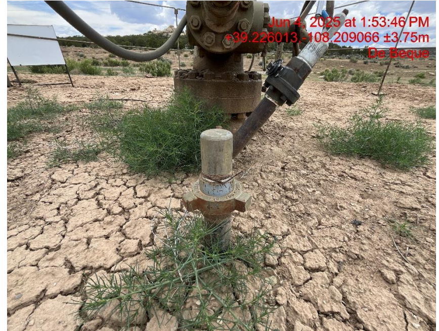
Photo # 7715 Intermediate Casing valve is buried/not in compliance with CECMC rules
