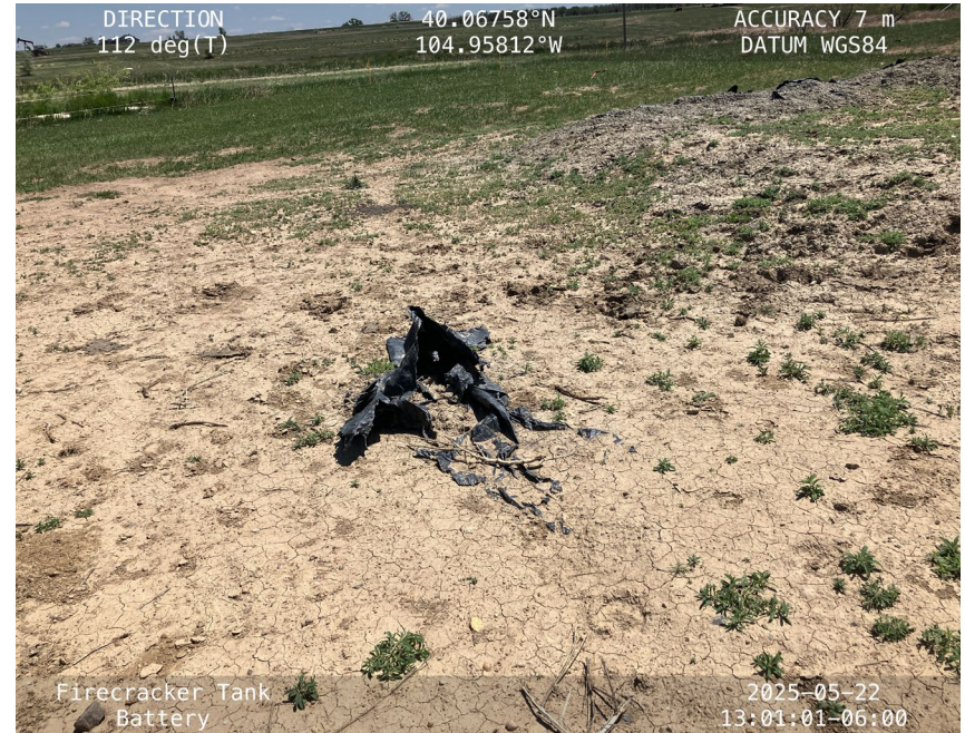
Torn liner at the stockpile
