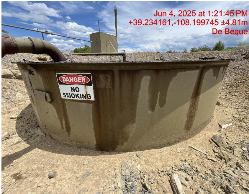
Photo # 7680 Staining on side of tank
