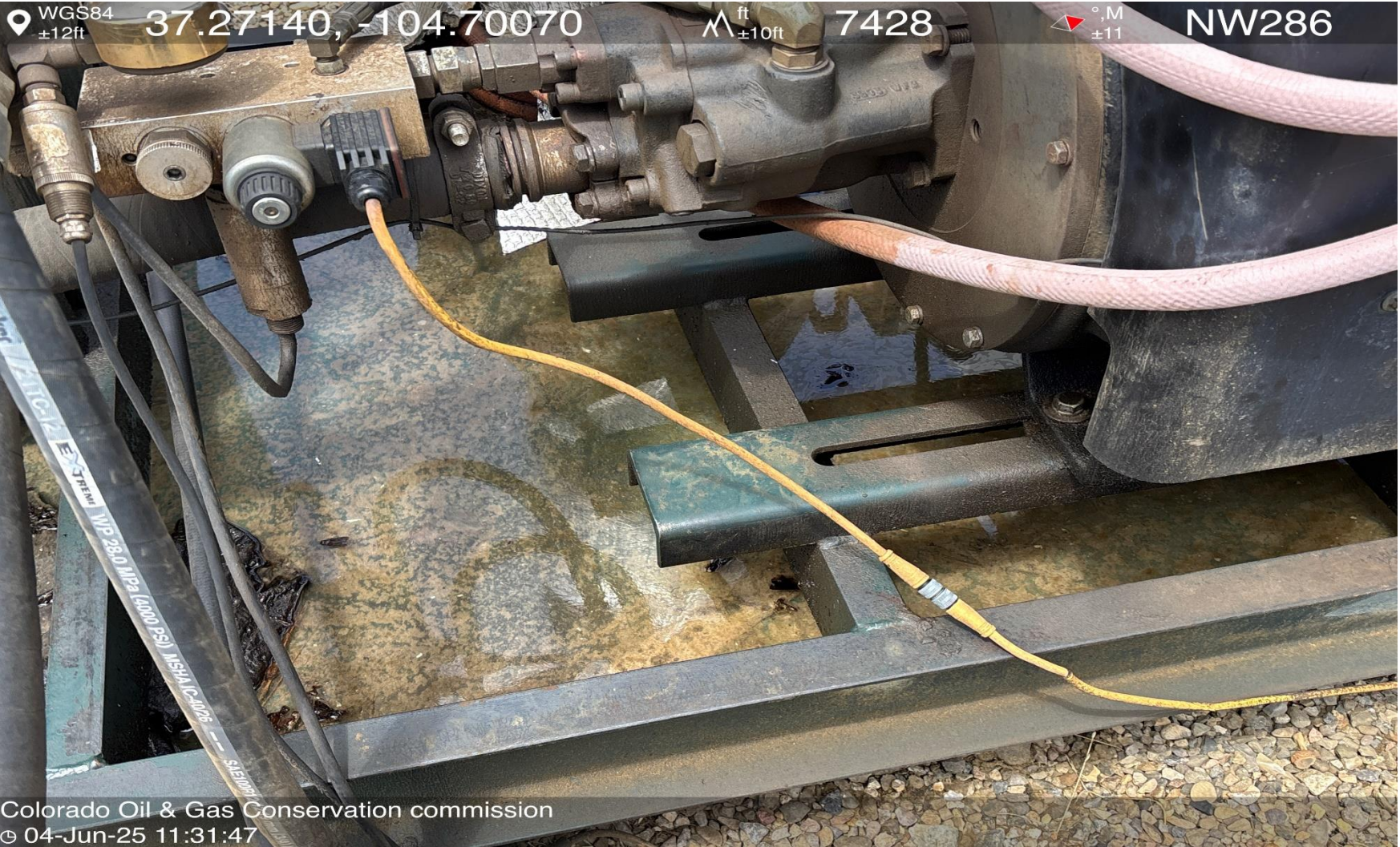
PHOTO 7: OILY WASTE INSIDE PRIME MOVER ENGINE SKID. DRAIN OILY WASTE REPAIR ALL LEAKS AND REMOVE IMPACTED SOIL PER RULE 1002..(2).D & 1002.f.(2)B, Comply with general provisions of the oil and gas act for wildlife protection AND SB-181. CA DATE 6/5/2025.
