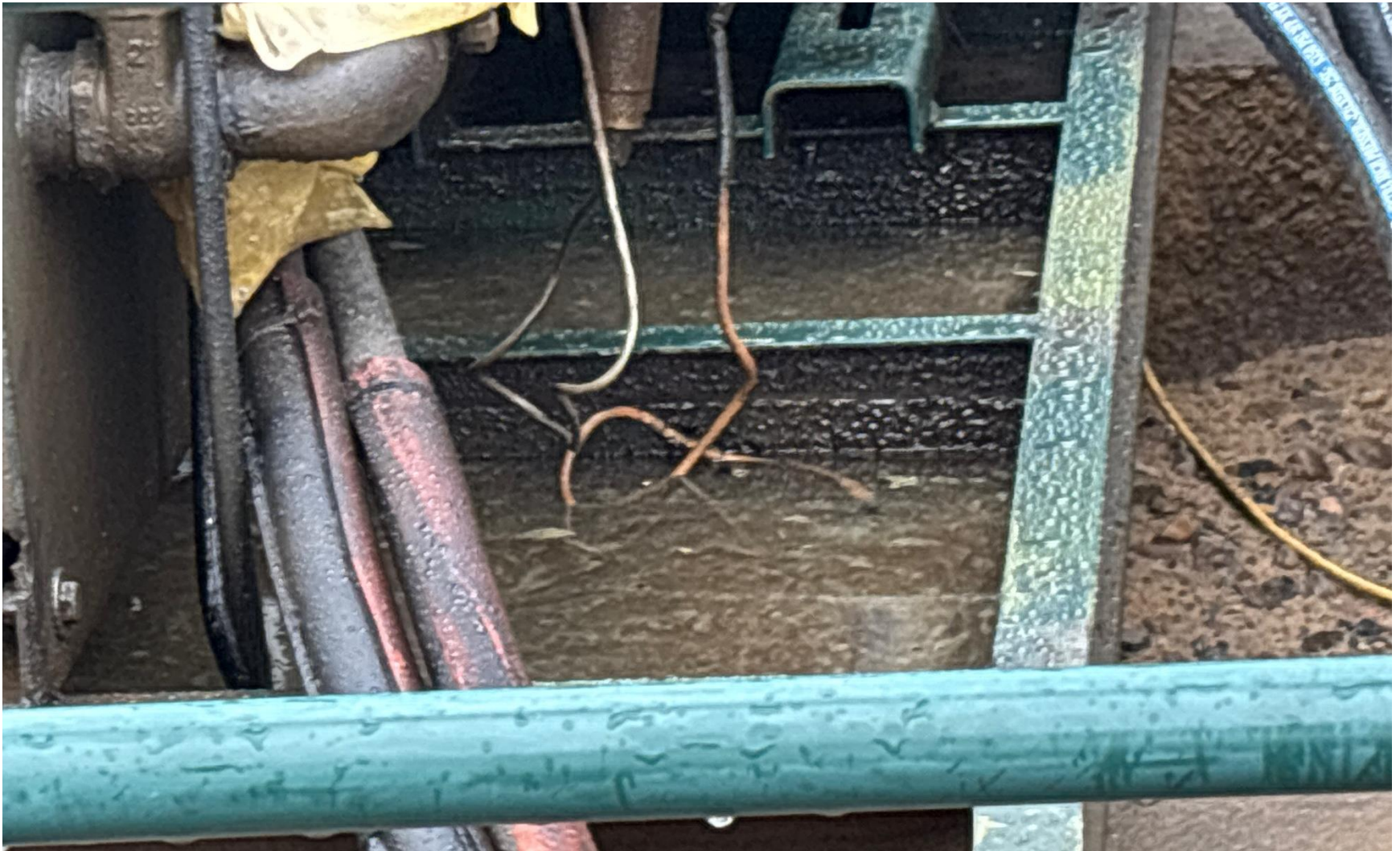
PHOTO 4: OILY WASTE INSIDE PRIVE MOVER ENGINE SKID. DRAIN OILY WASTE REPAIR ALL LEAKS AND REMOVE IMPACTED SOIL PER RULE 1002..(2).D & 1002.f.(2)B, Comply with general provisions of the oil and gas act for wildlife protection AND SB-181. CA DATE 6/3/2025.
