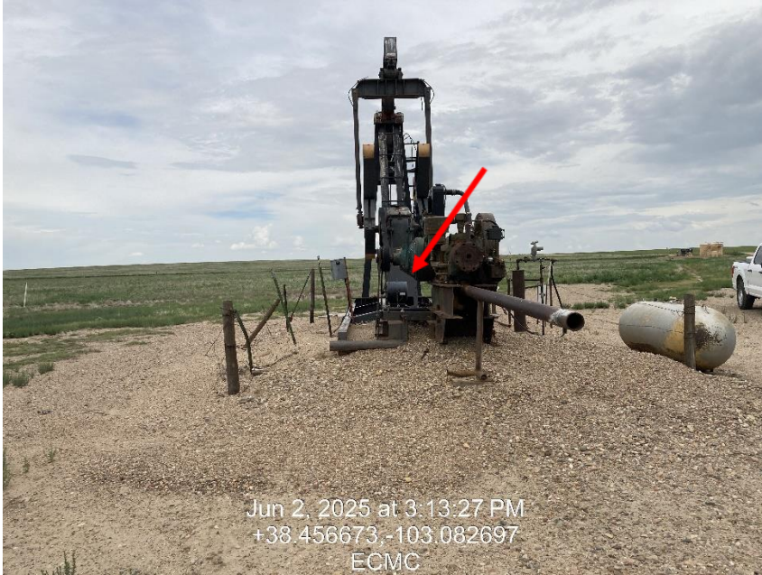
Photo 3 – Impacted soils at rear of pumping unit
