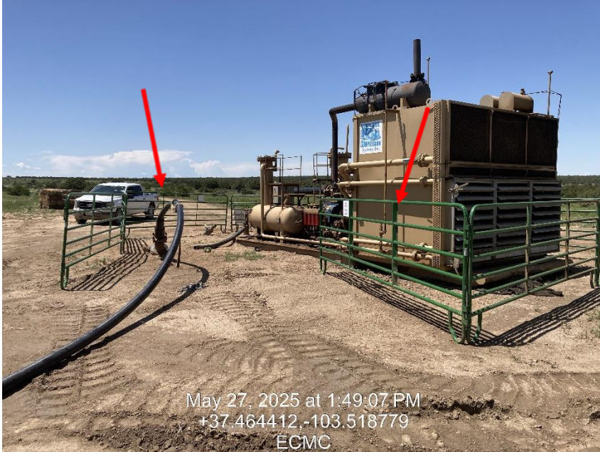
Photo 3 – Machine Guarding not maintained
