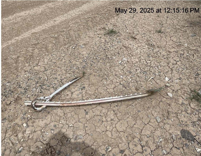
Photo # 4531 Improperly marked deadman
