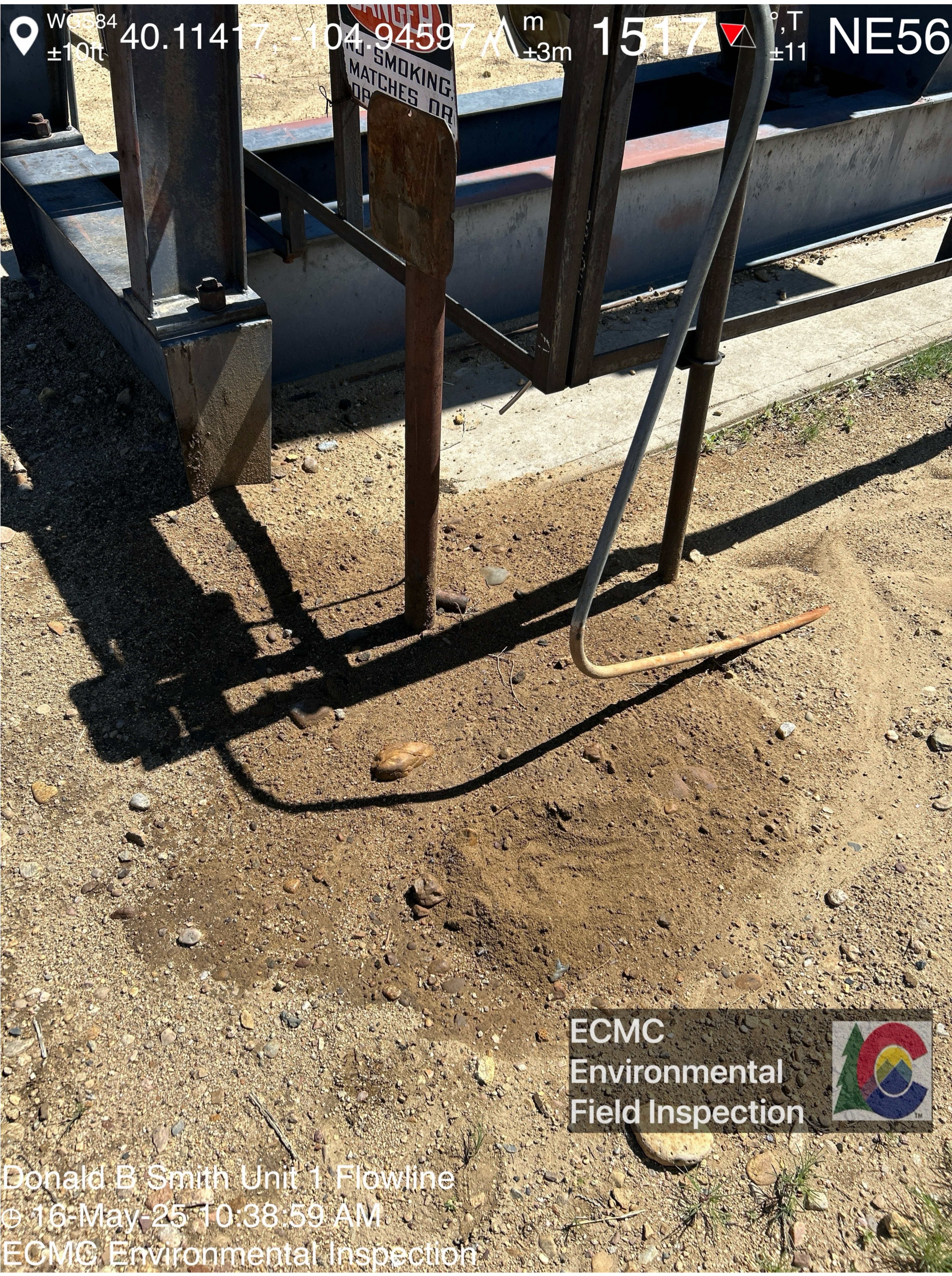
A strong petroleum hydrocarbon odor was observed when the stained soil was disturbed.
