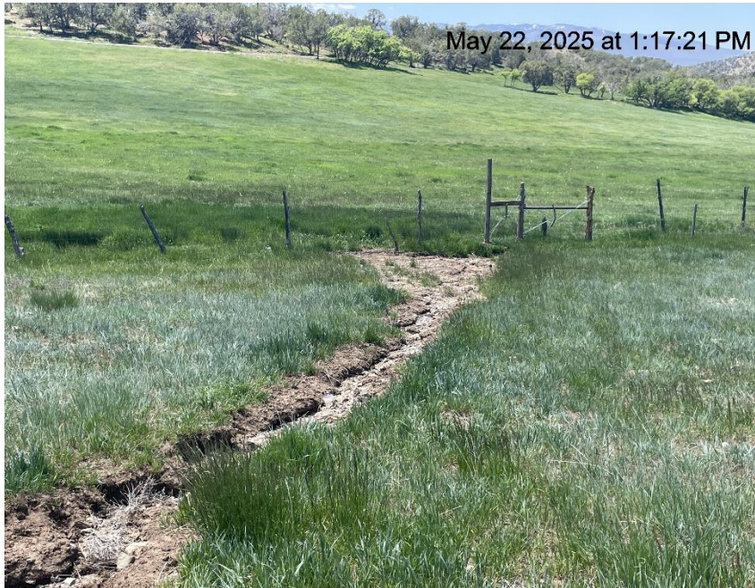
Photo # 2485 Failure to minimize erosion & transport of sediment off location/insufficient BMP's
