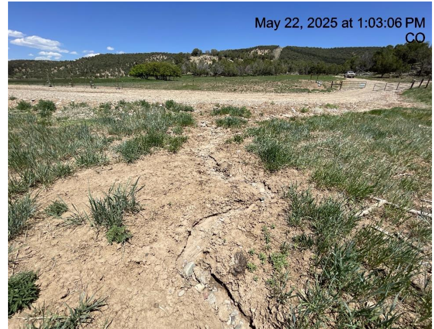
Photo # 2478 Failure to minimize erosion & transport of sediment off location/insufficient BMP's
