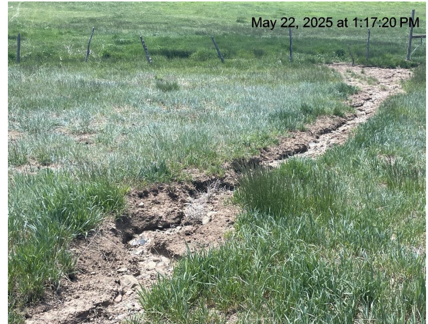
Photo # 2484 Failure to minimize erosion & transport of sediment off location/insufficient BMP's
