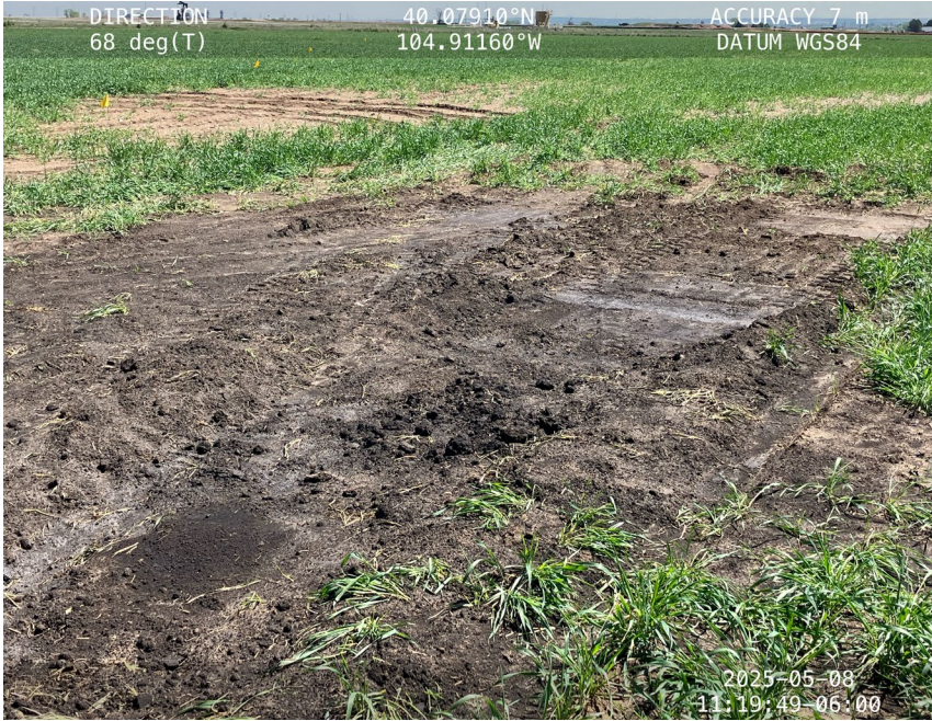
Spill with visible dark staining and hydrocarbon odor
