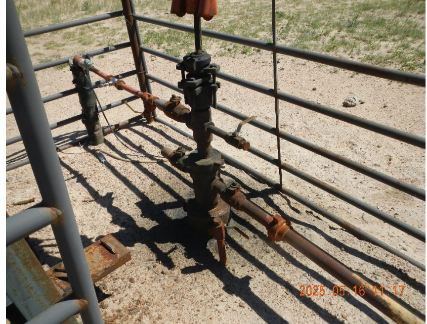
2. View of wellhead. Note staining around Wellhead.
