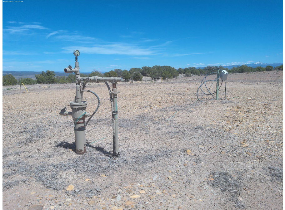
Fossil Federal #9 API 05-113-06076 Converted to water well
