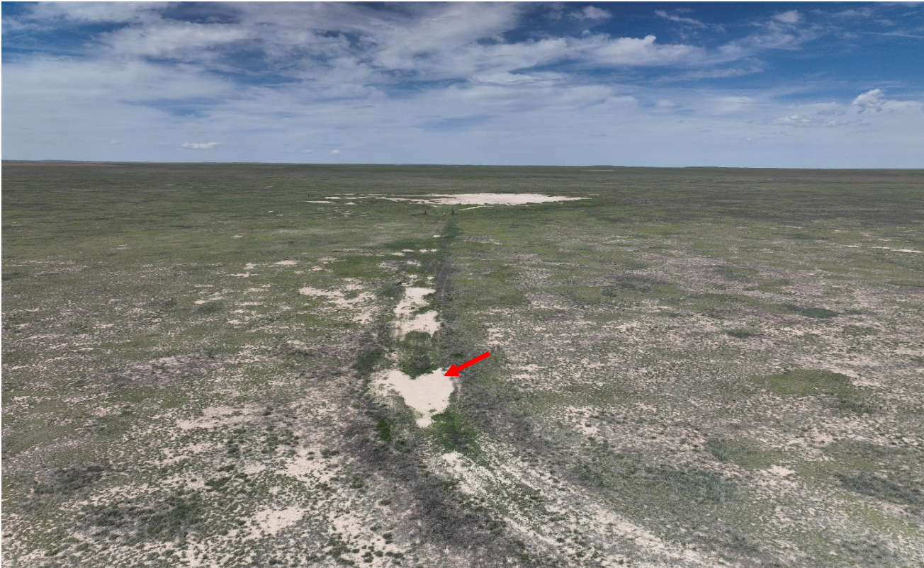
Photo 1. Drone aerial photo facing north along the access road and toward the location. There are areas of the access road that have not established vegetation shown at red arrow.
