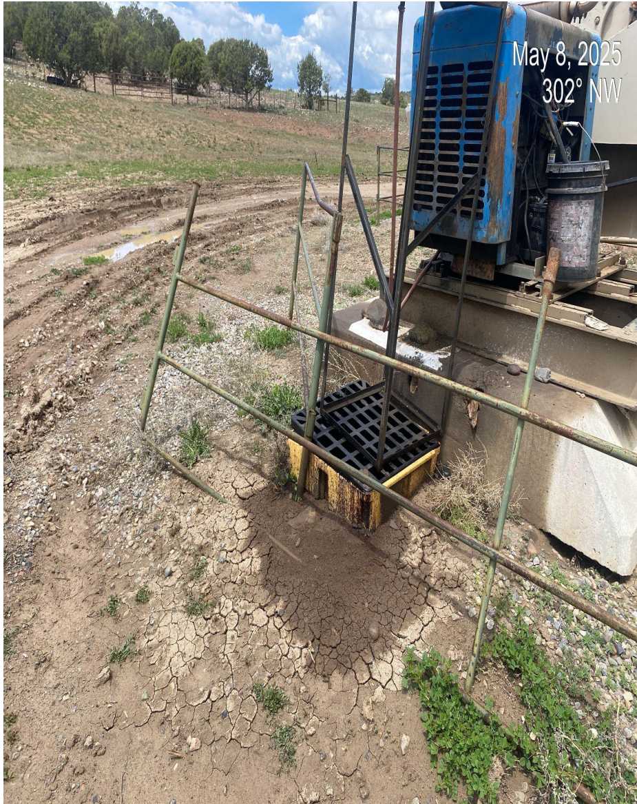
Photo 3. Stained soils at lube tank secondary contaminants.
