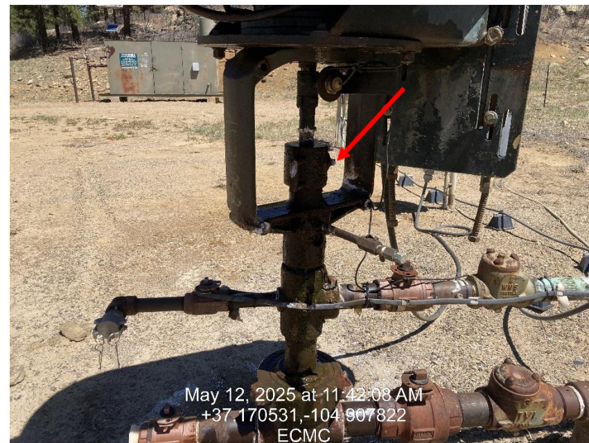
Photo 4 – Leaking packing
