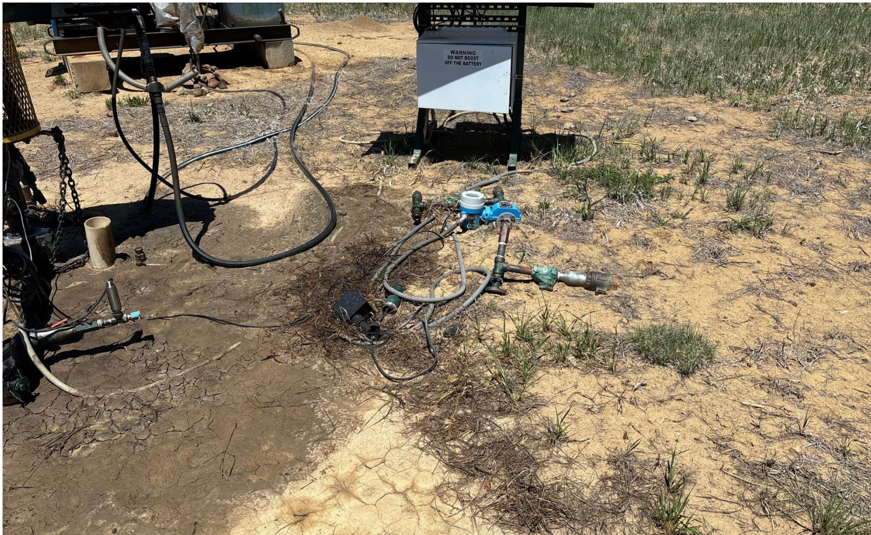
PHOTO 4: UNUSED EQUIPMENT LEFT ON LOCATION (MISCELLANEOUS PIPES AND METER, TELEMTRY EQUIPMENT DOES NOT APPEAR TO BE CONNECTED). REMOVE UNUSED EQUIPMENT PER RULE 606. CA DATE 5/22/2025
