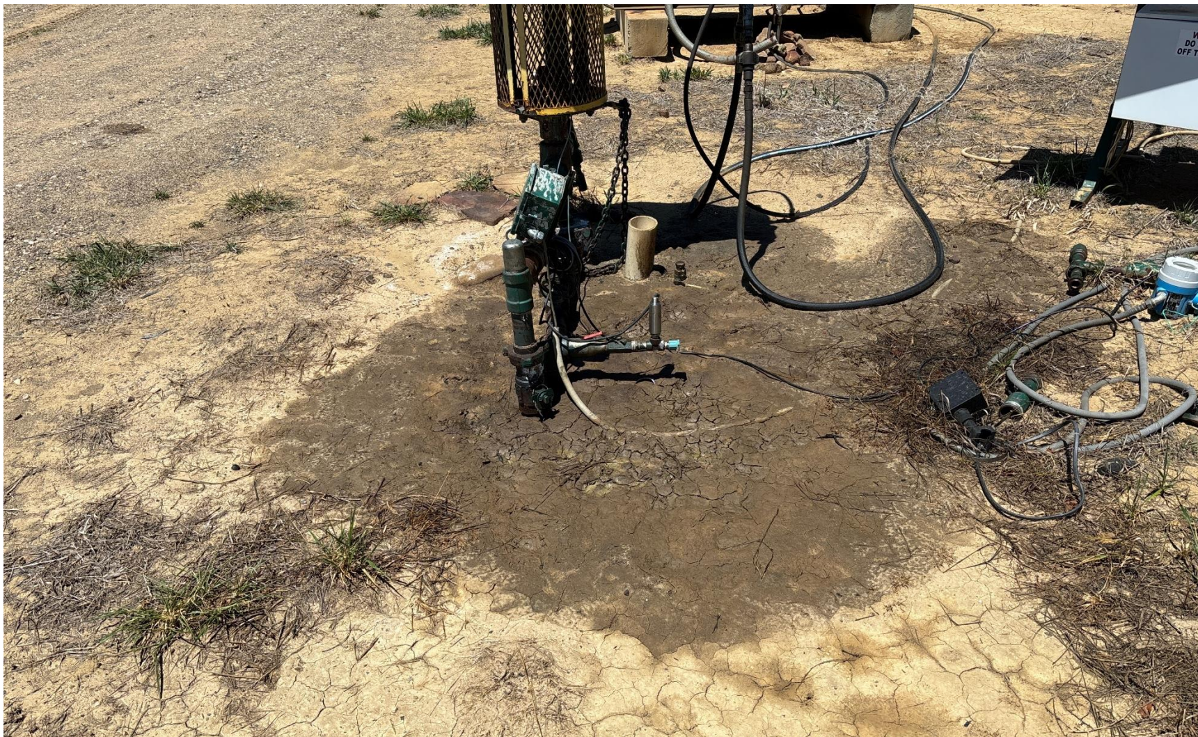
PHOTO 5: AREA OF IMPACTED SOIL AROUND WELLHEAD APPEARS TO BE LEAKING HYDRAULIC HOSES AND DRIVEHEAD. Conduct maintenance on equipment, cleanup stained material and review self inspection processes. COMPLY WITH RULE 1002,(2).D. CA DATE 5/22/2025.
