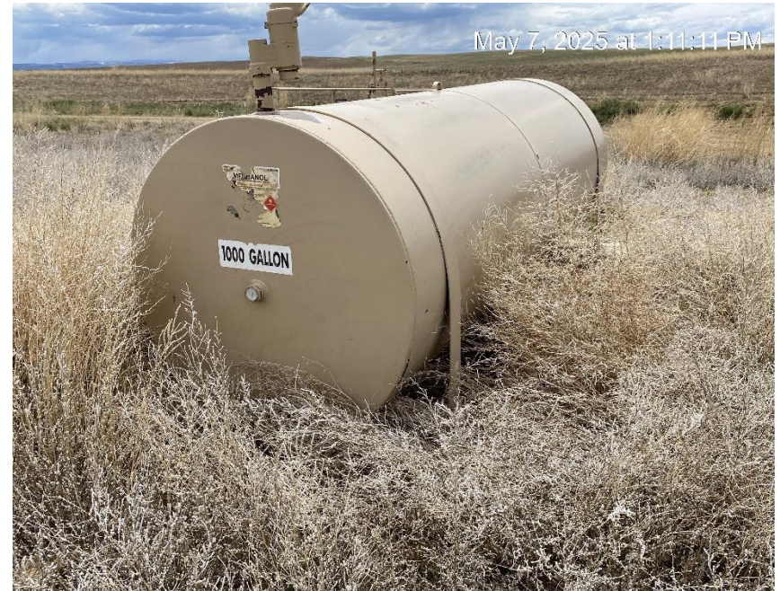
Unused equipment. Berm inadequate. Weeds.
