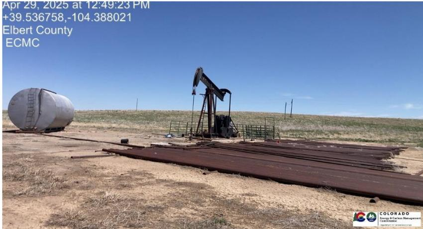
**Pic 3 tubing and tank needs to be removed from location**
