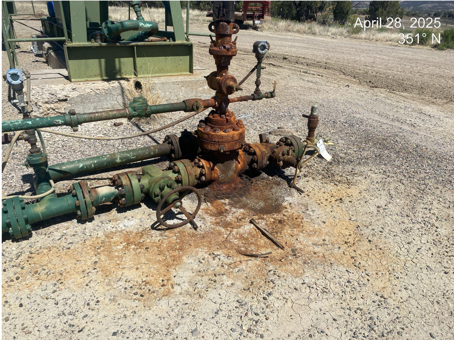
Photo 2. Stained soils observed at wellhead.
