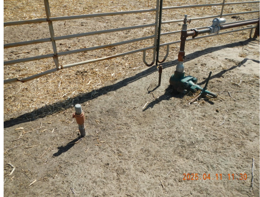
2. View of wellhead and Flowline Riser.
