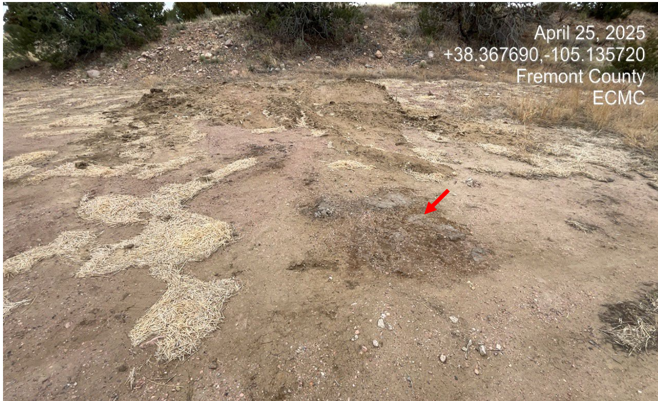
Photo 6. The oil stained soils still remain at the location. Impacted soils need to be excavated and removed.
